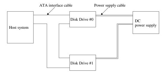
Figure 3.9 Cable connections
